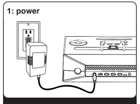
Attach AC adaptor cable to DC jack on back of the iD84 and plug the other end into a wall socket.
